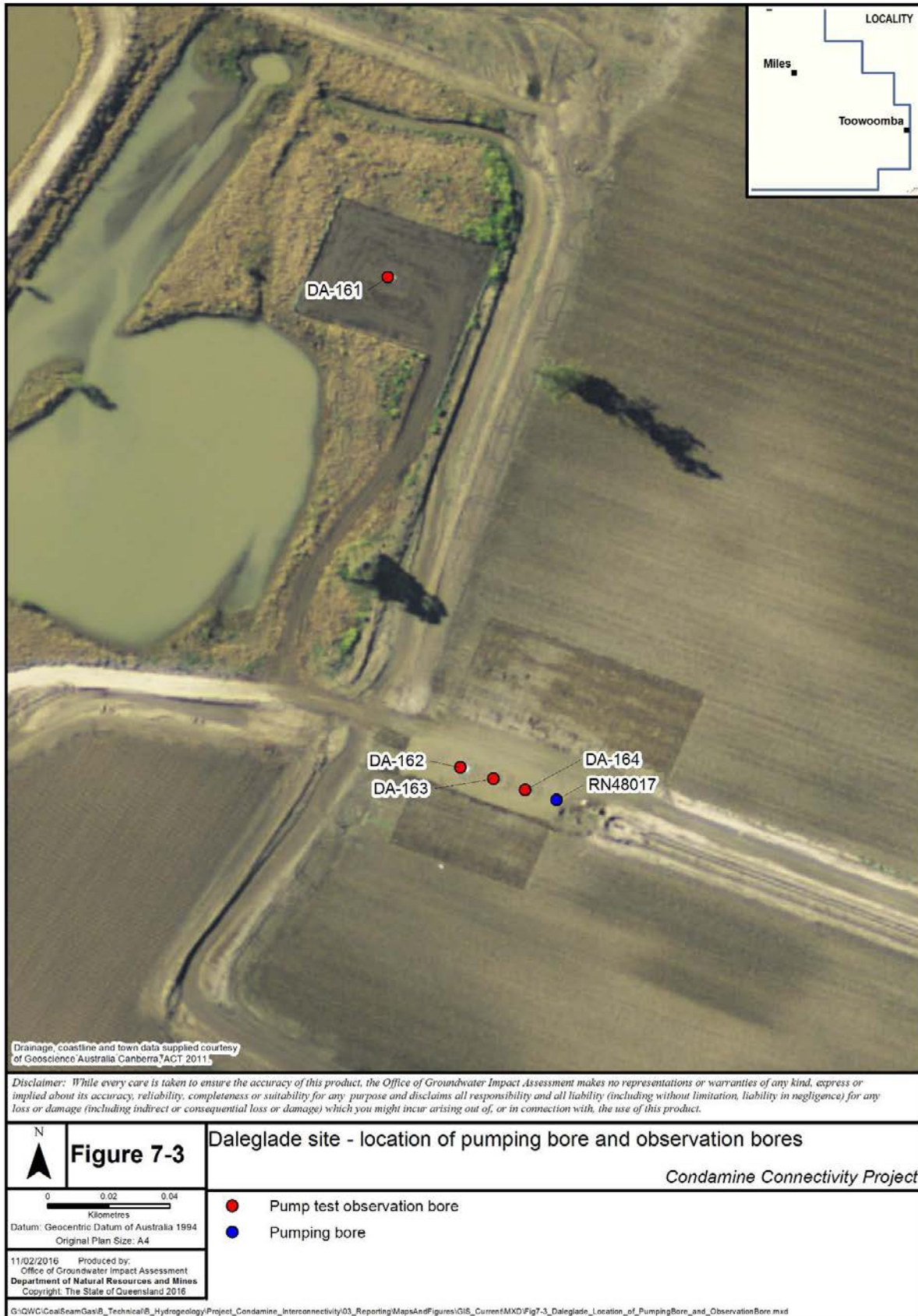
Figure 7-3 Daleglade site – location of pumping bore and observation bores
